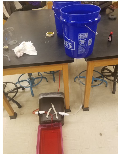
FIG. 5: The setup is very simple which helps with rapidly testing t-junctions. Each test took only around 30 minutes. Not pictured here is the camera used to photograph the dashed area during tests.
